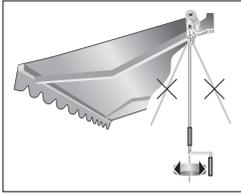
Turning direction to extend: Right (clockwise).
